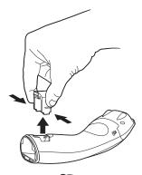
2. Remove the battery and end cap.
