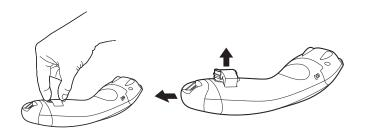
2. Remove the battery and end cap.
